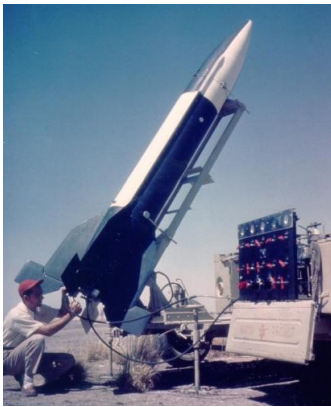
Rare color photo of a NATIV missile being prepared for launch from the Holloman AFB missile test range.
